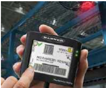
RD35 Handheld Remote Display Used for programming
