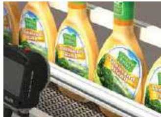
Match Sensor — Compares a part to a reference to determine if there is a match
