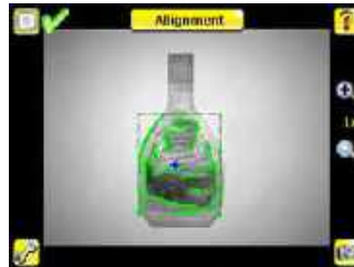
Match Sensor — Compares a part to a reference to determine if there is a match
