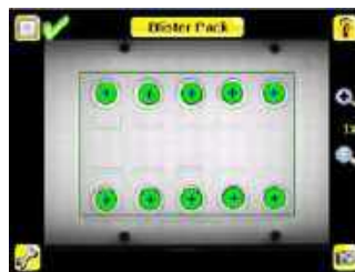
Area Sensor — Detects whether a particular feature (features) are present
