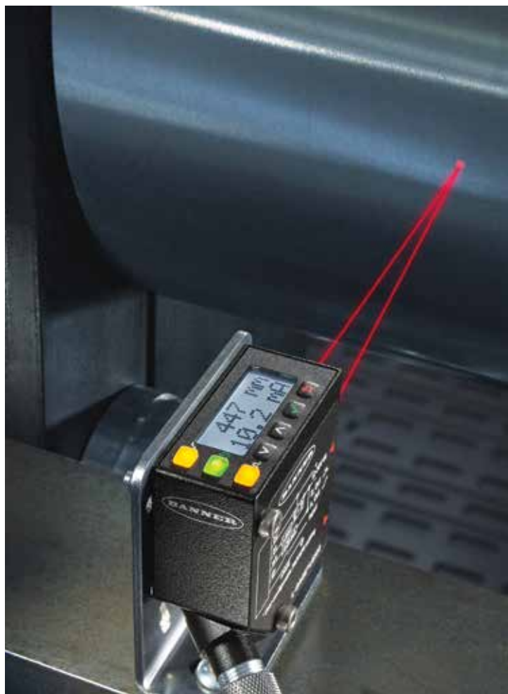
Monitoring sheet metal roll diameter
